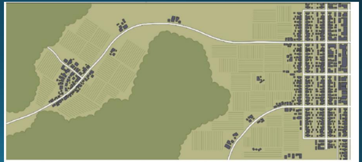
Clustering homes is safer because the agricultural land (shown as striped rows) provides a protective buffer. This pattern of development also is easier to defend from fire and requires fewer fire suppression resources. Source: Fire Mitigation in the Wildland Urban Interface.
