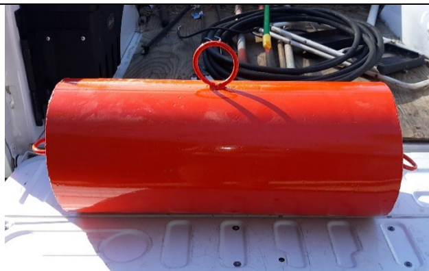
Figure 4. Refurbished pipe buoy.
